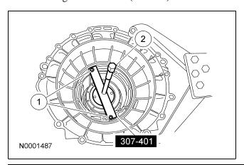
74. **NOTE:** Align the disc holes on special tool with the slot in gauge bar for correct measurement.
